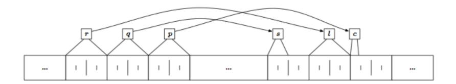
An example of a schematic view of memory. The smallest division represents one 8-bit memory location.
