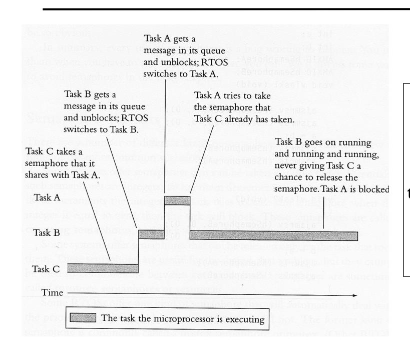
A high-priority task (Task A) that wants the semaphore then has to wait until Task B gives up the microprocessor: Task C can't release the semaphore until it gets the microprocessor back.
