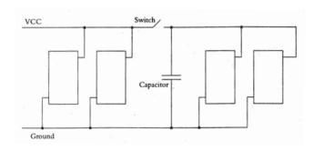
but the circuitry on the right side gets turned on and off, using the switch, from time to time in order to save some power. The capacitor shown in the middle of the diagram is to cushion the voltage when the switch is closed. What is wrong with this design? What are the symptoms most likely be? How should it be fixed?
