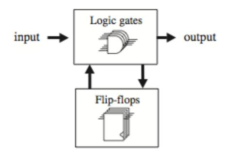
Notice that in this case the output might change when the input changes (asynchronous output).
