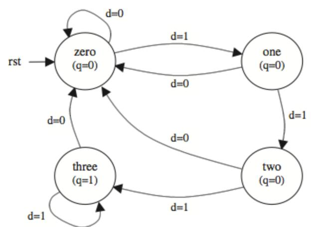
We want to design a circuit that takes as input a serial bit stream and outputs a 'l' whenever the sequence "III" occurs.
